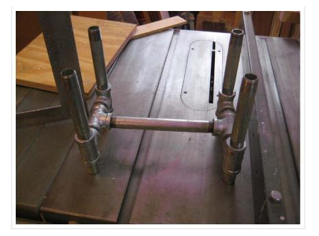
After I got all the pipes screwed together – remember, joints nice and tight – and by that I mean you have to bump them with a hammer to move them – I put the stool leg assembly on my table saw to adjust the legs so that the stool sat flat. Keep at this until there is no wobble.
