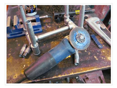
The 2 1/2" nipples for the lower legs were longer than I wanted, so I used an angle grinder with a cut-off blade to shorten them by an inch. This lowered the cross brace to a level that I found pleasant to the eye.
