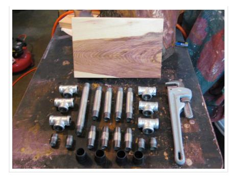
You will need the piece of wood you want for the seat and a variety of steel pipe fittings and nipples. For this stool I used 1/2" galvanized pipe – 6 each T-fittings, 4 each 5" nipples for the upper legs, 4 each 2 1/2" nipples for the lower legs, an 8" nipple for the cross brace and 4 each 3/4" crutch tips for the feet. You need a pipe wrench as it is really important to get the joints tight.
