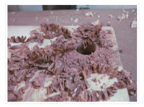
The holes are all drilled so that the bottoms of the holes (the tops of the legs) are a uniform distance below the top of the seat. For this stool, I stopped the holes 5/8" below the seat surface. Make sure all four holes are evenly bottomed.
