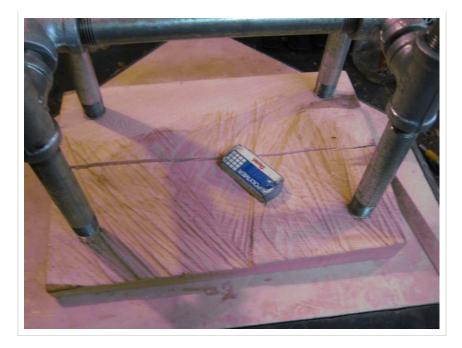
With the leg assembly tight, squared and sitting flat, I laid the stool top up side down and marked the locations where the legs will join the top. This piece of wood varies a lot in thinckness so I had to be certain the leg assembly was square to the flat upper surface of the stool seat before I marked the spots I will drill.
