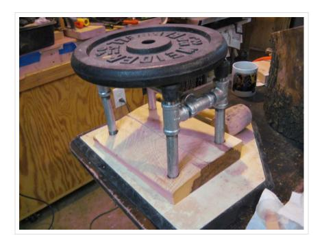
I slipped the crutch tips onto the lower legs and checked the fit of the legs into the holes. Carefully measure the height of the stool on all four corners with the stool standing upright to ensure that the four legs stack to a uniform height. I had to grind one leg as I just couldn't tighten it as far as the other three legs. Once the height is true, mix up about 2 ounces of 5
