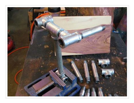
Just start twisting the pipe pieces together – working from the cross brace out. I used a flat machinist's vise to help me hold the pieces while torquing things down.
