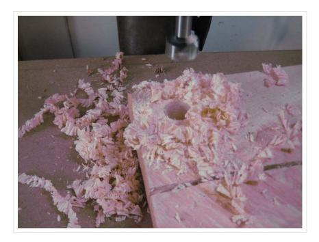
The 1/2" galvanized pipe is 0.84" outside diameter. I used a 7/8" (0.875") Forstner bit to drill holes into which the legs will fit.
