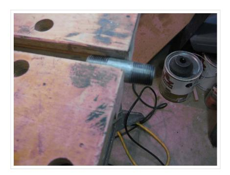
To cut the short nipples, I just clamped them in my WorkMate – any secure clamping arrangement will work. Just cut the nipples to length and then use the angle grinder to smooth the exposed (unthreaded) ends.
